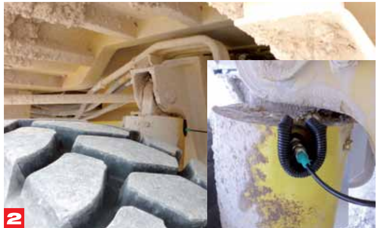
Load sensor, one for each front suspension
