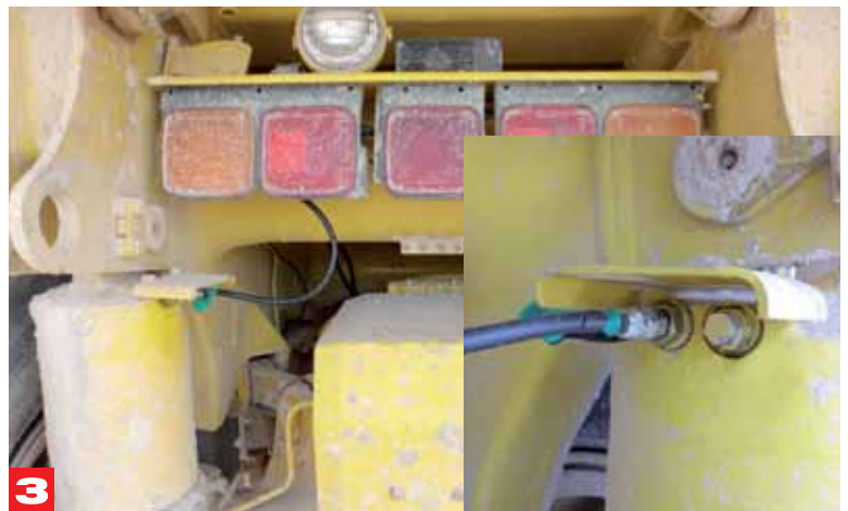
Load sensor, one for each rear suspension
